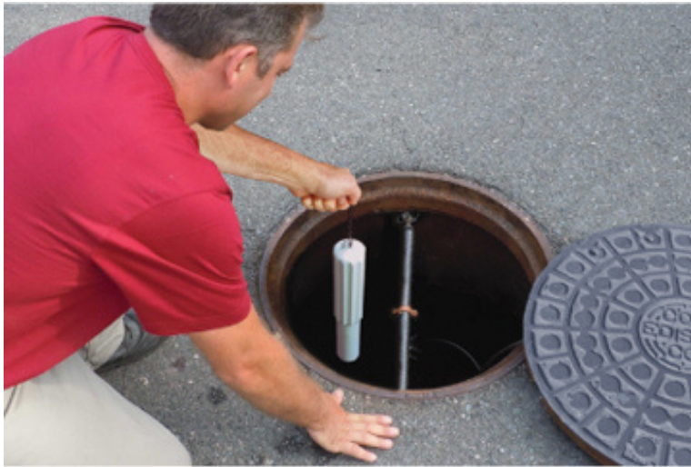
Figure 2: iTracker sensors, weighing just under 2 lbs. are installed without the requirement for confined-space entry
